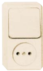
Combination socket-outlet without earth 16 A, AC 250 V, CEE 7 norm sheet XIII Combined with two-way switch 10 A, AC 250 V.
