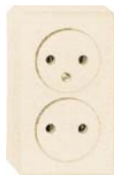
Double socket-outlet without earth 16 A, AC 250 V, CEE 7, norm sheet XIII With screw terminals.
