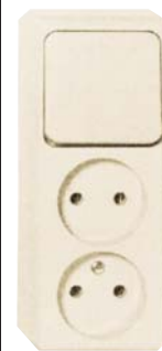
Combination double socket-outlet without earth 16 A, AC 250 V, CEE 7, norm sheet XIII Combined with two-way switch 10 A, AC 250 V.
